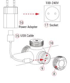
During charging, a charging icon appears on the right of the battery icon, and the LED indicator on the device is red. When the indicator turns green, it indicates that charging is complete.
