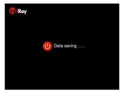
interface "Data saving ..." is displayed. When the data is saved, the display turns black and the device is off. **During the saving data**, do not disconnect it from the power source, otherwise, the data cannot be saved.
