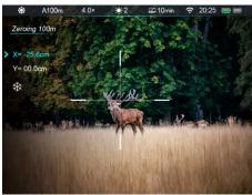
Move the reticle by rotating the Controller (7) until the reticle matches the point of impact. To switch the reticle movement direction between X axis and Y axis, press the **Controller (7)** briefly.
